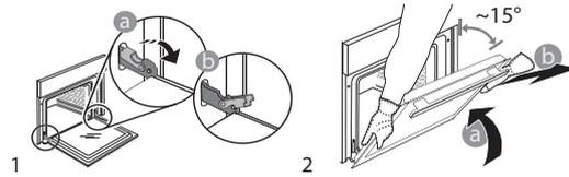
Refit the door by moving it towards the oven, aligning the hooks of the hinges with their seating and securing the upper part onto its seating. Lower the door and then open it fully. Lower the catches into their original position (3): Make sure that you lower them down completely. Apply gentle pressure to check that the catches are in the correct position.
