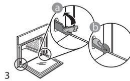
Try closing the door and check to make sure that it lines up with the control panel. If it does not, repeat the steps above: The door could become damaged if it does not work properly.
